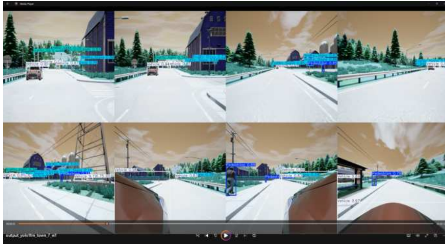
Figure 6.16: Real-time object detection using YOLO11m in Town07 of CARLA simulation under default weather conditions. The results demonstrate the model's generalization to a completely unseen environment.
