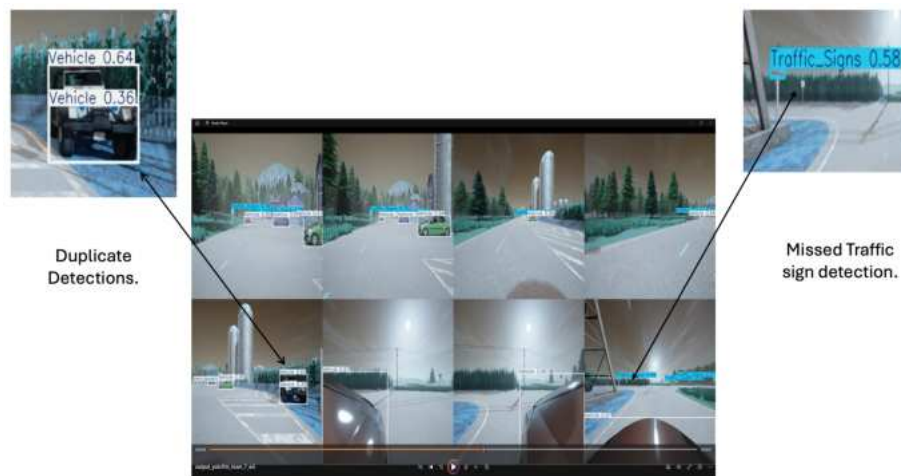
Figure 6.19: Real-time object detection using YOLO11m in CARLA simulation. The frame highlights duplicate detections and missed long-range traffic signs.
