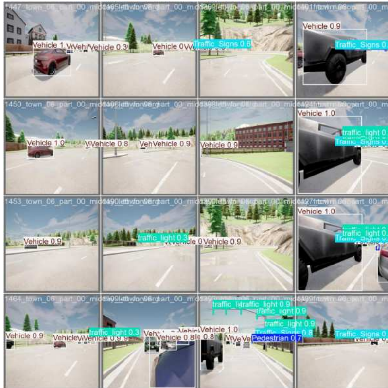
Figure A.5: Predicted labels visualization for test dataset batch 1 during YOLO11m model inference. This figure shows how the model predicts objects in the test dataset.
